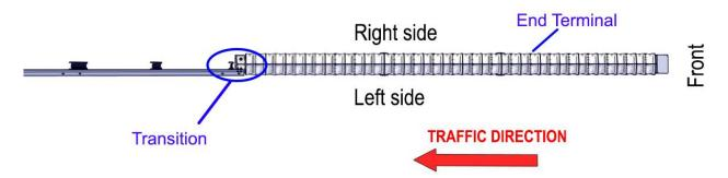
Fig. 2: Top view of the End Terminal connected to the barrier.
