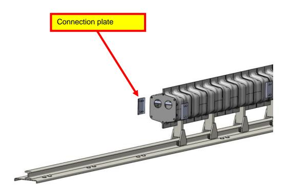
Fig. 24: Removing procedure of the modular bay
