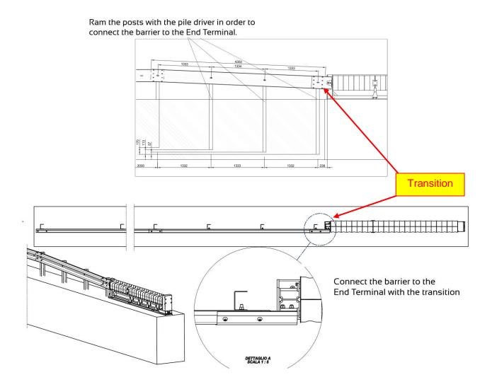
Fig. 20: Connection of the barrier to the End Terminal – top and side view.
