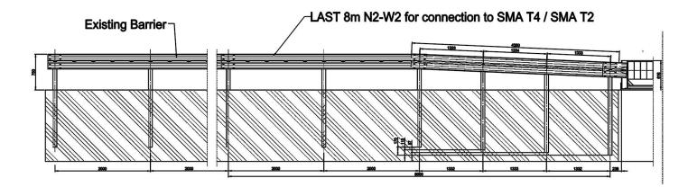
Fig. 21: Connection of the barrier to the End Terminal - complete view.
