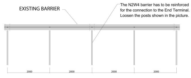
Fig. 19: Side view of the barrier before the installation of the End Terminal
