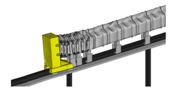
Fig. 22: SMA T 4 frontally impacted
