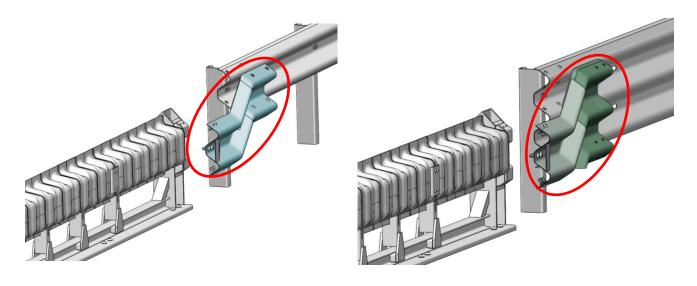
Fig. 16: Example of transition to double beam barrier
