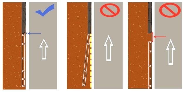
Fig. 5: Top view of the drilling template positioning compared with possible errors.
