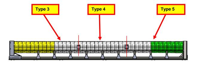
Fig. 28: Collapsible beam sections SMA T 4
